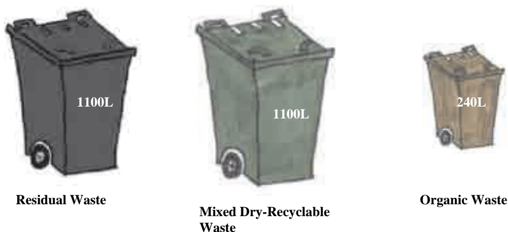
Figure 9.1. Suggested bin capacity ratio for residual, mixed dry-recyclable and organic waste (not drawn to scale).
