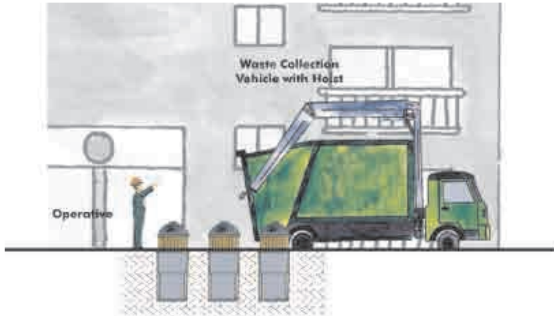
DESIGN 3: Deep Storage Bins - Elevation View
